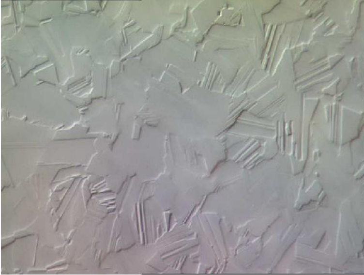
Surface image of pCVD sample (Courtesy Element6 )
