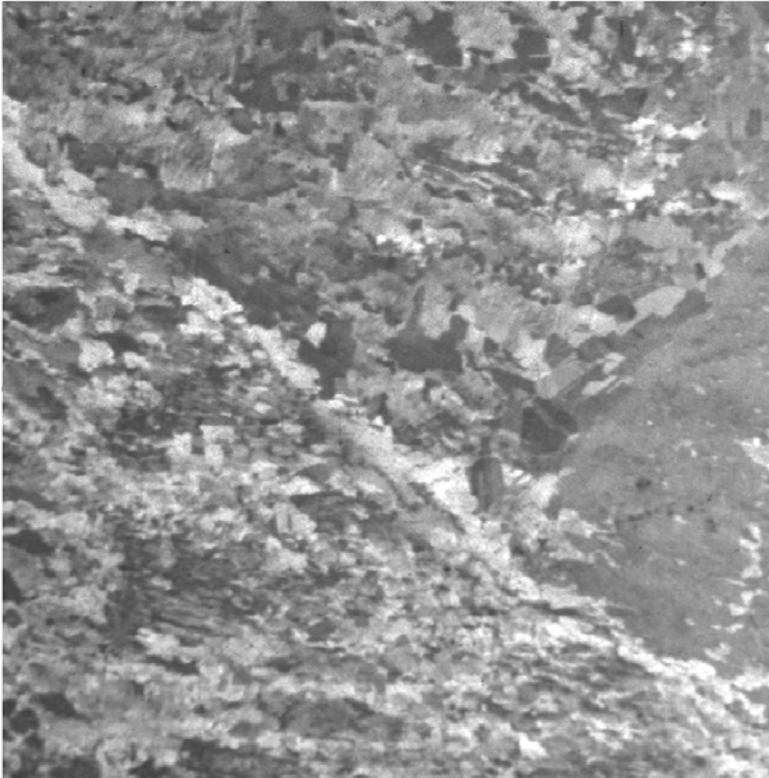
266 nm image of LCLS copper cathode, 30 x 30 microns
