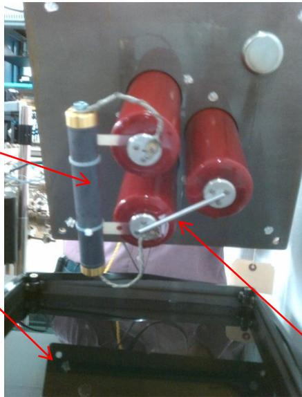
100 MΩ Conditioning Resistor
