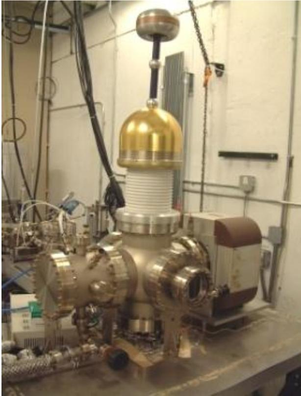
Stainless Steel and Diamond-Paste Polishing Good to  $\sim 5\text{MV/m}$  and 100kV.
