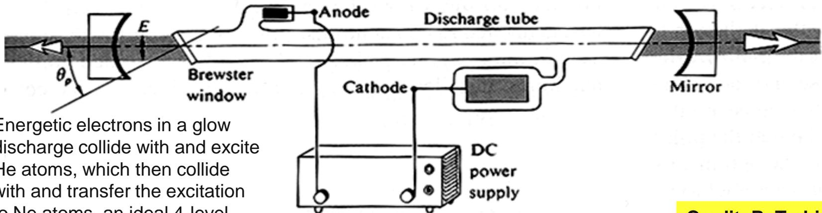
Energetic electrons in a glow discharge collide with and excite He atoms, which then collide with and transfer the excitation to Ne atoms, an ideal 4-level system.
