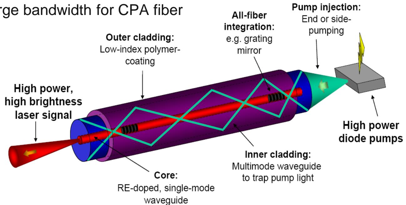
Rare-earth-doped core converts multimode pump energy to high brightness, *diffraction-limited*, signal beam
