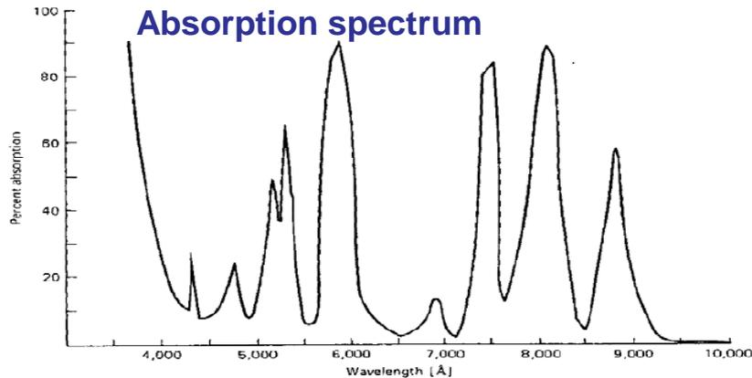
Fig. 2.9. Absorption versus wavelength of Nd: glass. (Material: ED-2; thickness: 6.3 mm)
