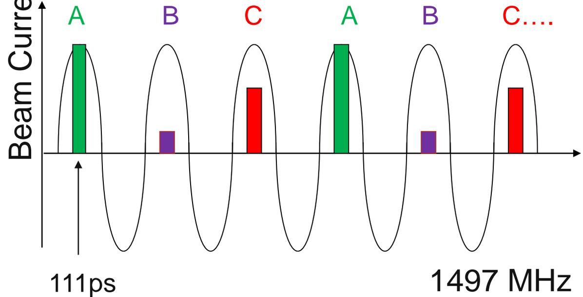
Extracting DC beam, very wasteful, most of the beam dumped at chopper. Need ~ 2mA from gun to provide 100uA to one hall. Gun lifetime not good enough.....yet.
