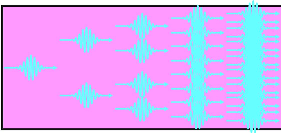
This is the essence of the laser. The factor by which an input beam is amplified by a medium is called the **gain** and is represented by  $G$ .
