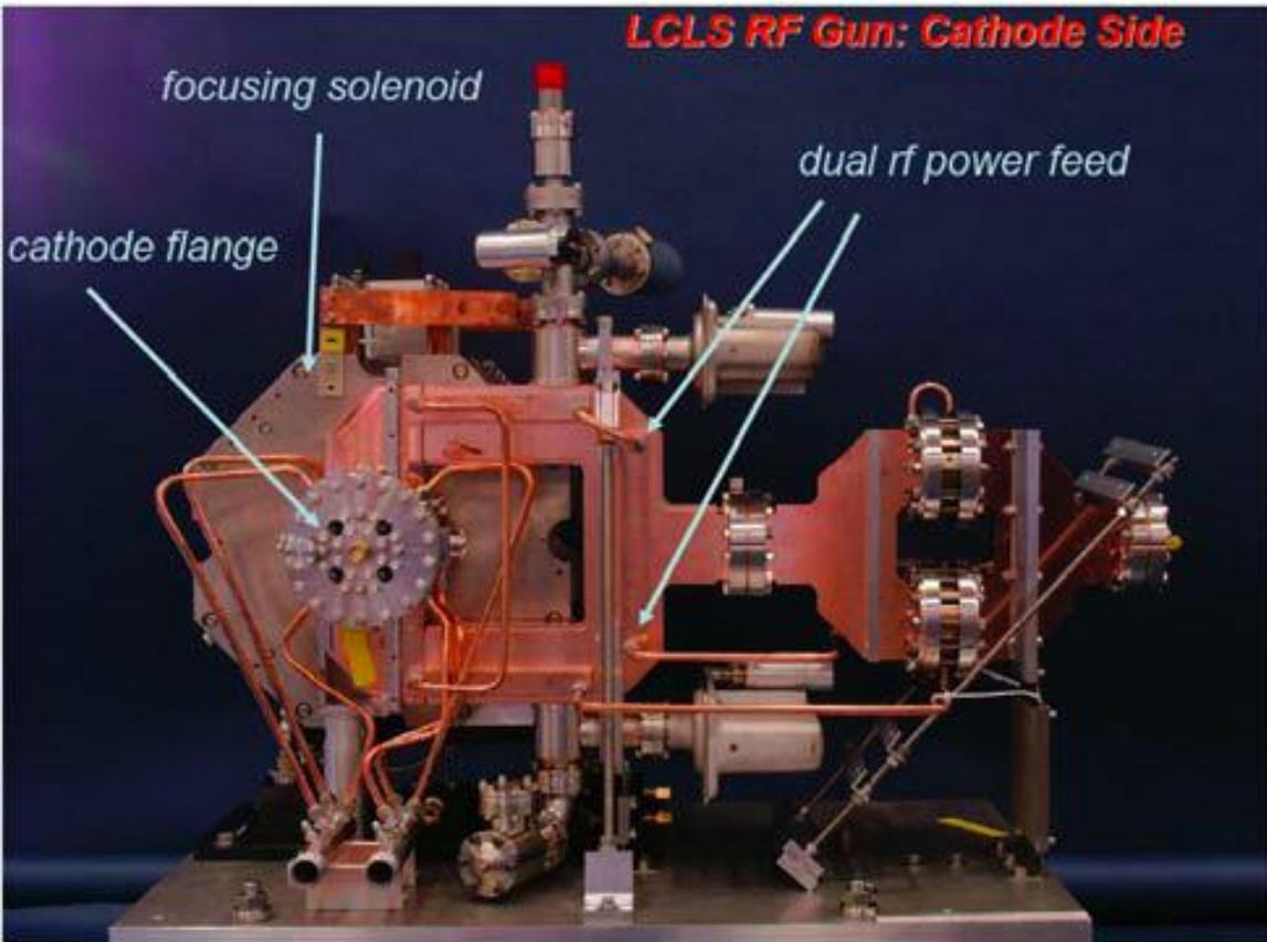
The LCLS RF photoinjector is the state-of-the-art technology with a Cu cathode. It generates electron beam with  $0.7 \mu\text{m}$  emittance.
