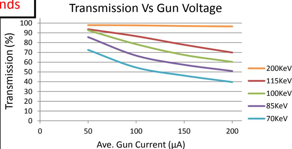
Message: Beam quality, including transmission, improves at higher gun voltage
