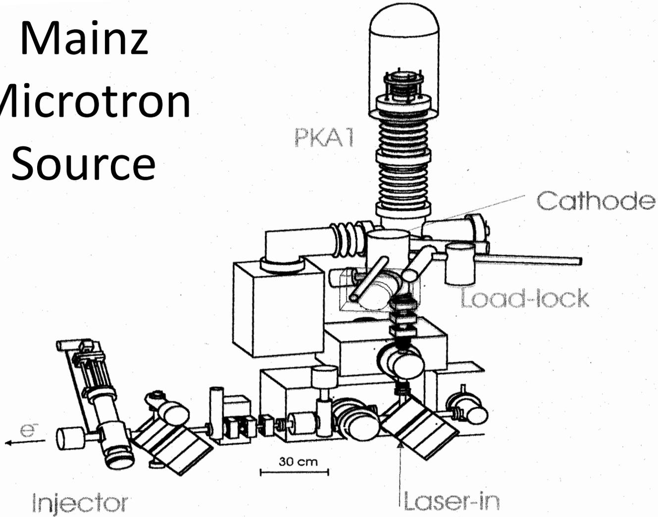
Polarized electron source Installation
