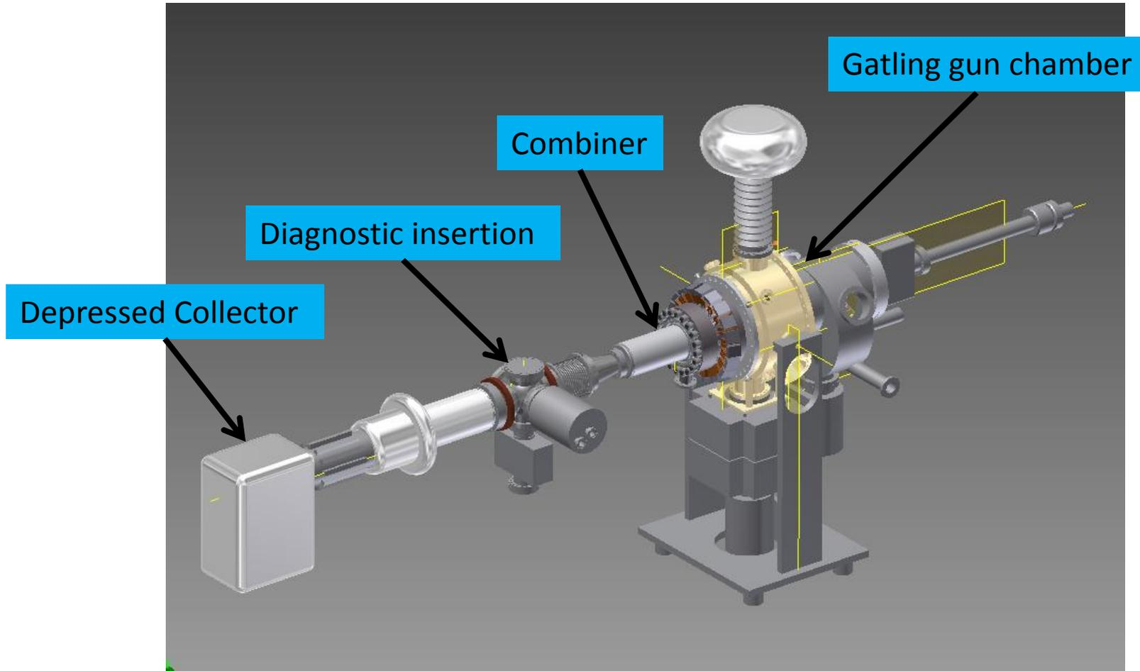
Depressed Collector can reduce the HV power supply current, reduce radiation.
