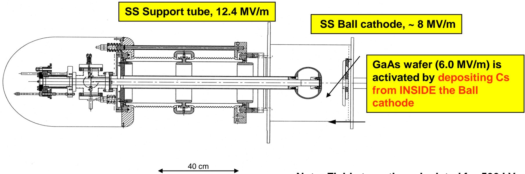
Note: Field strengths calculated for 500 kV
