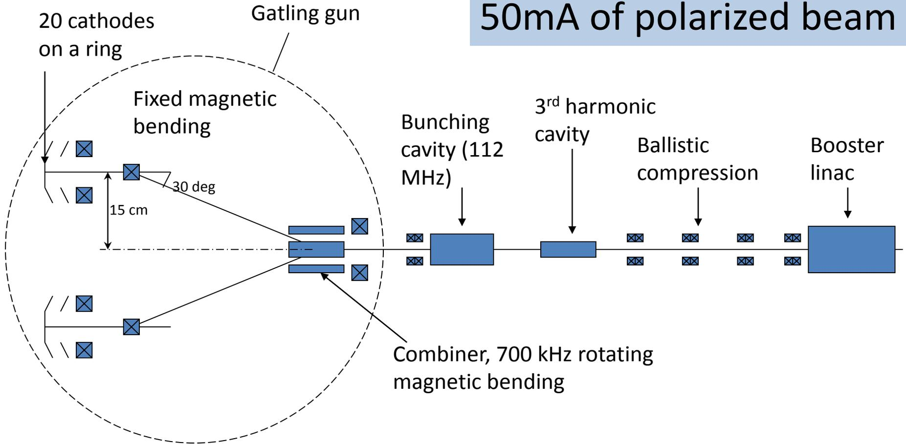
The lowest requirement for the “Gatling gun” is to verify that the cathode lifetime is not affected running at multiple (2) cathode mode.
