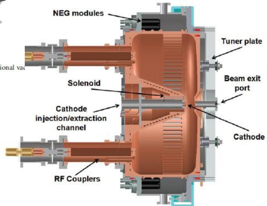
Figure 7: Low frequency, normal-conducting CW gun developed at LBNL [12, 13].
