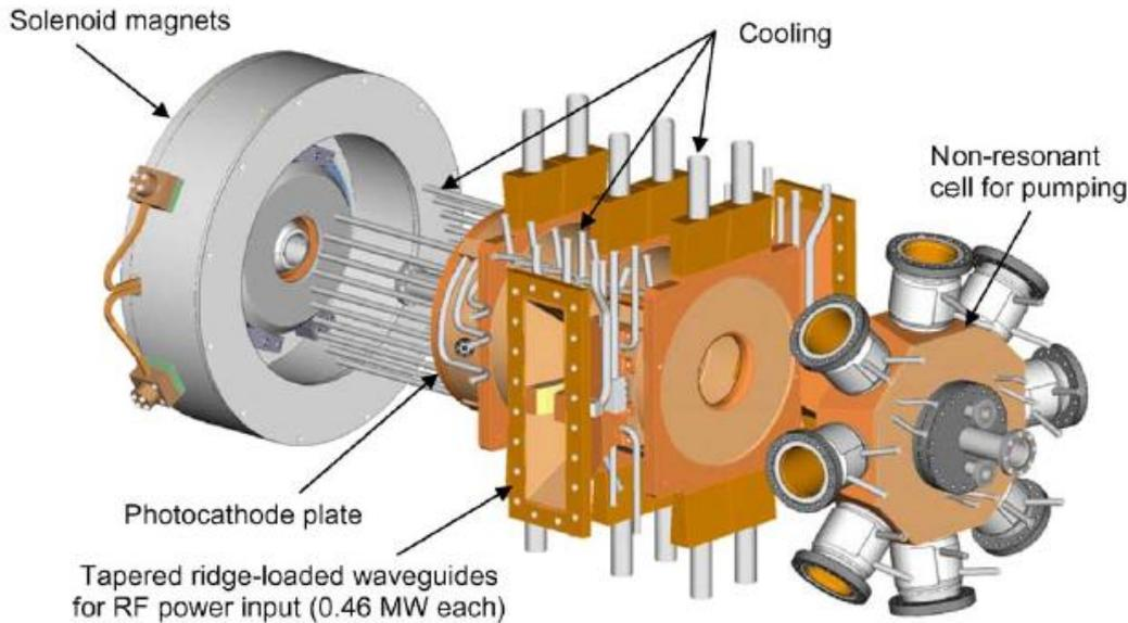
view of the  $2\frac{1}{2}$ -cell NCRF gun being fabricated by AES for LANL. The non-resonant cell provides additional vac
