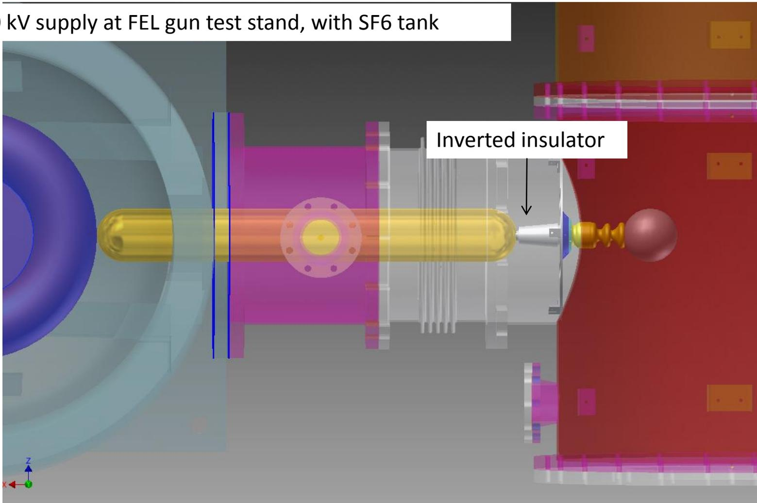
Learn to apply high voltage without breakdown, dielectric plug inside insulator,
