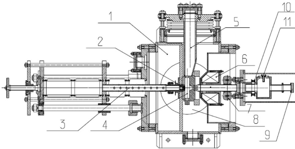
Figure 1: The scheme of RF gun prototype. 1 - activation chamber, 2 - photocathode assembly, 3 - manipulator, 4 - accelerating cavity, 5 - waveguide, 6 - focusing lens, 7 - transverse corrector, 8 - working chamber, 9 - vacuum window for laser beam, 10 - ceramic insulator, 11 - the cavity for bunch length measurement.
