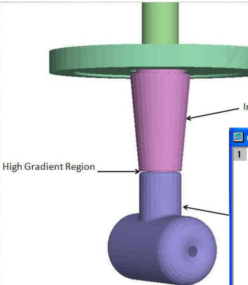
Our design has one region of “unintended” high gradient – could be problematic.....exploring new designs via electrostatic modeling
