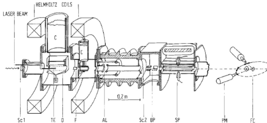
Fig. 3. Longitudinal section of electron source and polarization analyzer. *O* oven system, *F* Faraday cup, *AL* accelerating lens, *SP* spin precessor (Wien filter), *FC* foil carrier (details are not shown), *PM* photo-multipliers, *TE* test electron source, *BP* beam steering plates, *Sc*<sub>1</sub> and *Sc*<sub>2</sub> positions of scintillators for laser beam adjustment, *C* cold traps
