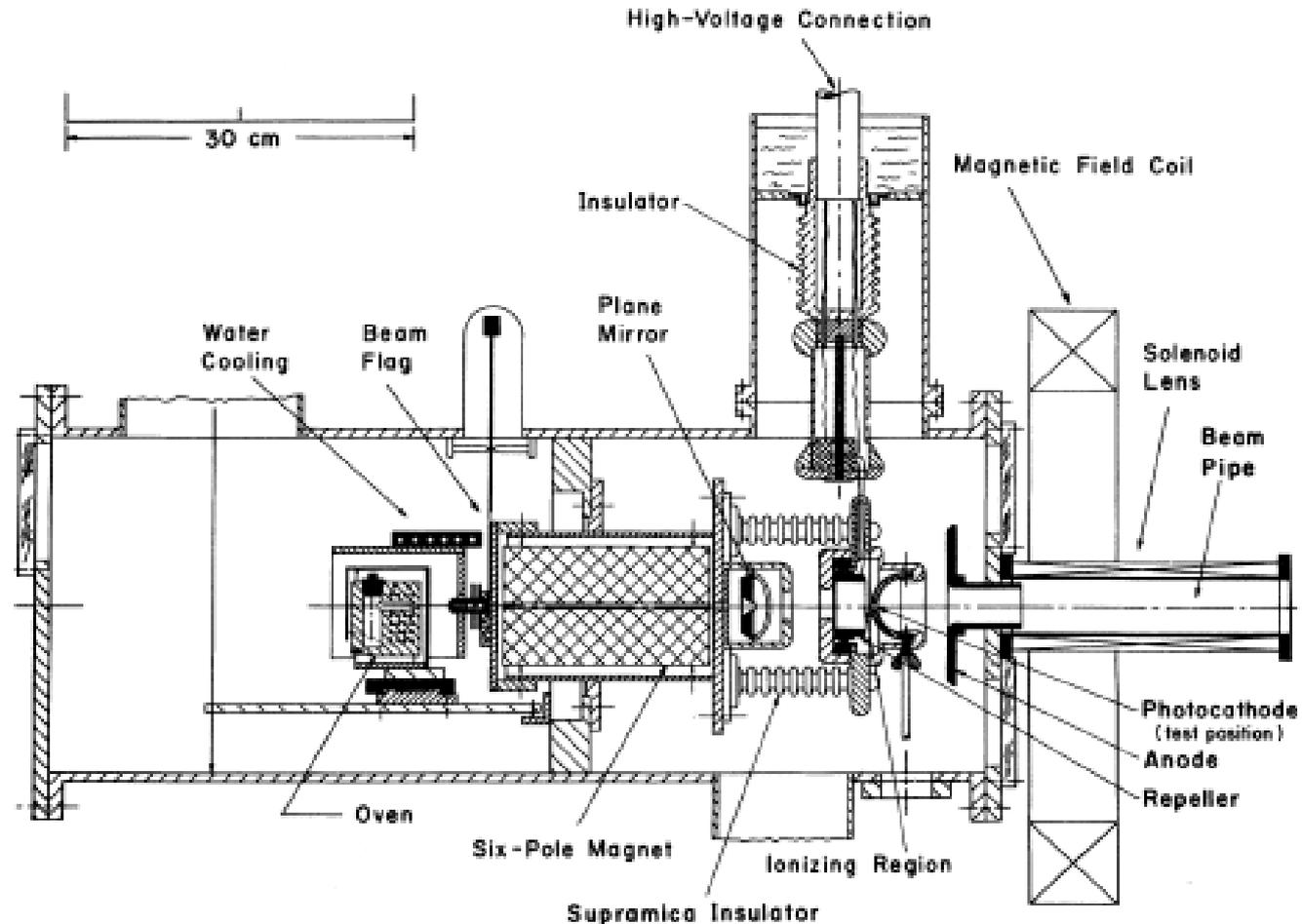
FIG. 18. Scale drawing of the polarized electron source assembly.
