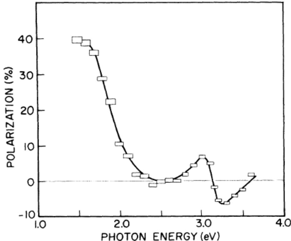
FIG. 6. Spectrum of spin polarization from GaAs + CsOCs at  $T \leq 10$  K [the same sample and conditions as curve (a) of Fig. 5]. Note the high value of  $P=40\%$  at threshold ( $\hbar\omega \sim 1.5$  eV) and positive and negative peaks at  $\hbar\omega = 3.0$  and 3.2 eV.
