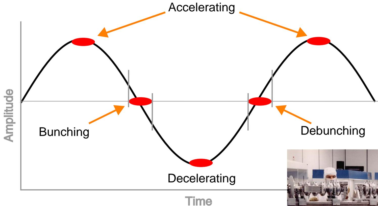
So only a portion of the RF cycle is good for accelerating e-beam
