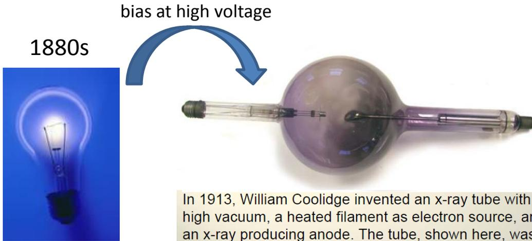
In 1913, William Coolidge invented an x-ray tube with high vacuum, a heated filament as electron source, and an x-ray producing anode. The tube, shown here, was produced in the 1920s by General Electric Corporation.
