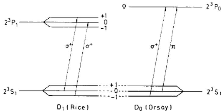
Fig. 2. Helium optical pumping process via  $D_0$  and  $D_1$  transitions.
