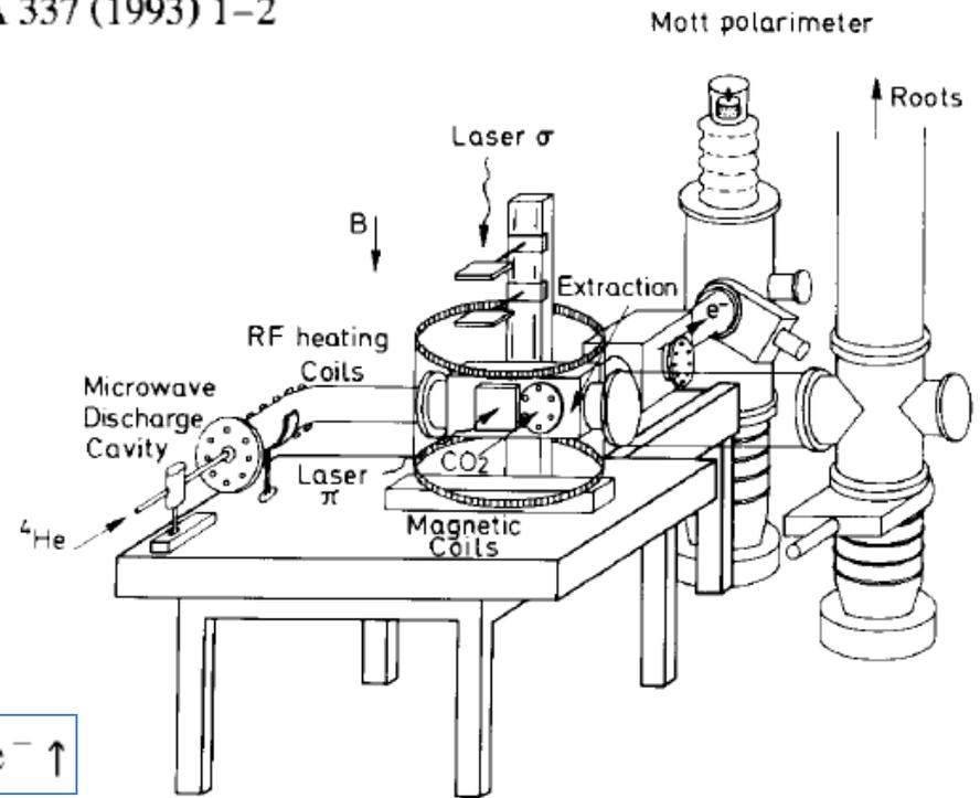
Fig. 1. Diagram of the Orsay source.
