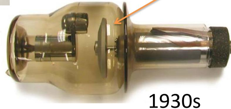
X-rays are generated when a DC electron beam, typically a few mA, strikes a tungsten target at 60-200 keV. e-Beam quality is not a big concern
