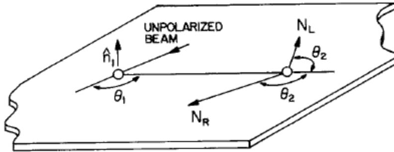
FIG. 1. Schematic diagram of a double-scattering experiment.
