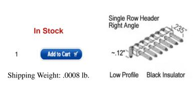
HWS4015 NUMBER OF PINS: 5 **1X5** SINGLE ROW BREAKAWAY **RIGHT ANGLE LOW PROFILE** HEADER .1"(2.54mm) CENTERLINE .025" SQUARE POSTS .235" MATING SIDE POST LENGTH **GOLD FLASH PLATING**
