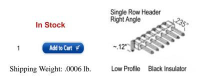
HWS10037 NUMBER OF PINS: 4 1X4 SINGLE ROW BREAKAWAY RIGHT ANGLE LOW PROFILE HEADER .1"(2.54mm) CENTERLINE .025" SQUARE POSTS .235" MATING SIDE POST LENGTH GOLD FLASH PLATING
