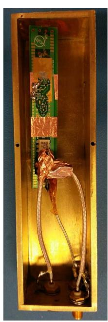
From top to botom, the first segment of copper tape covers the components on the back of the board, and soldered to ground on two points, although there is somo exposed copper underneath the tape that is connected by contact. There is a layer of Kapton tape on top the of the components being covered, keeping them from shorting.
