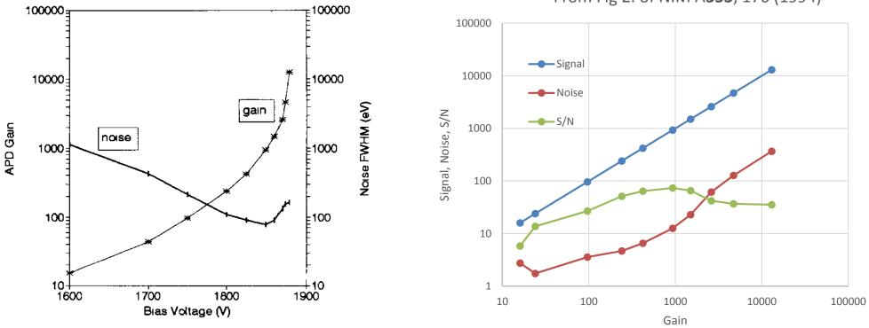
For gains < 500, the results are similar to those on slide 6 (tho better S/N at a given gain observed on slide 6), while for higher gains the noise rises more quickly with gain (excess noise factor F changes), the S/N drops.
