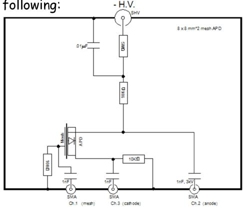
Three outputs are connected to scope via SMA cables.
