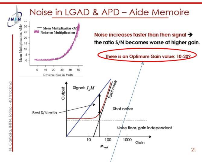
According to this argument it raises a series question about the application of APD to the fast timing: LGAD 10~20 gain is better than high gain APD (>100)<sub>2</sub>
