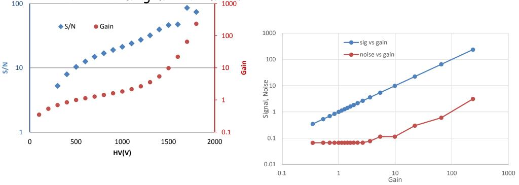
An optimum S/N value of 10-20 is not the case for an RMD APD. The baseline noise rises more slowly than linearly with gain, favoring operation at the highest possible gain.
