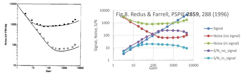
The noise during the signal is the rms width of the observed pulse-area distribution.
