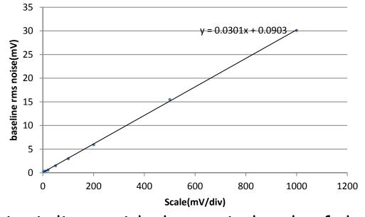
The rms noise is linear with the vertical scale of the scope.
