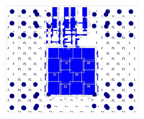
$4 \times 4$  APD array, made from 4 4-channel carrier boards.
