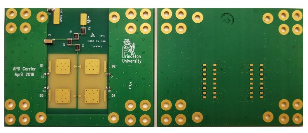
4-channel carrier board, for use with Penn ASICs. Designed by Stan Chidzik.
