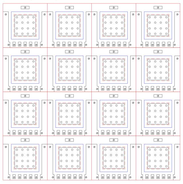
One APD on each of 4 tiling layers, Showing how 100% coverage is thereby obtained
