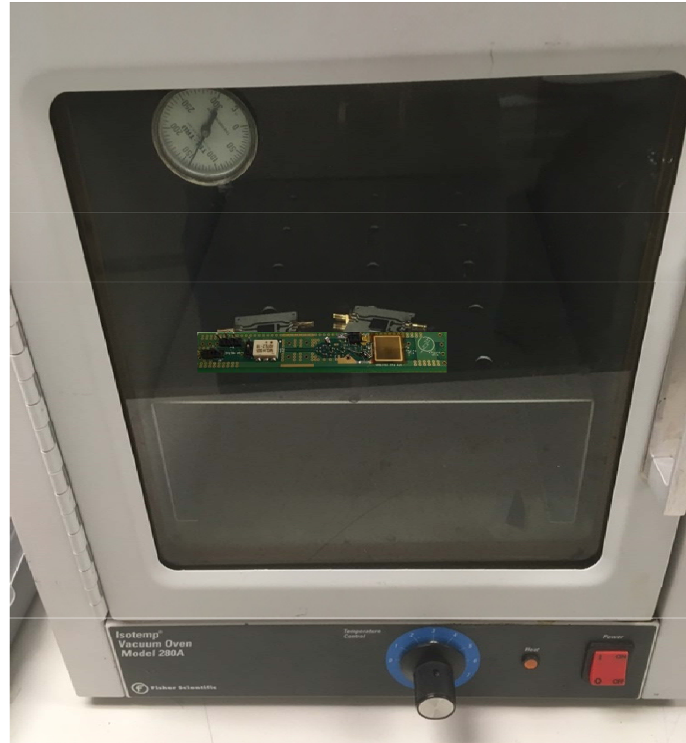
Cure Epoxy in Vacuum Oven 5 Minutes @ 150C
