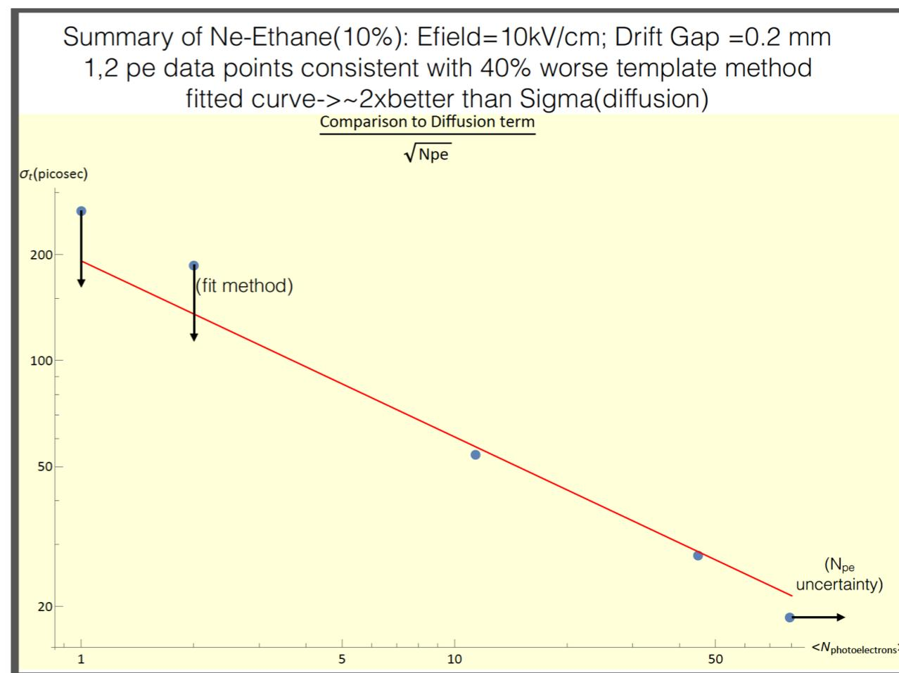
Technology tested on bench, can yield 30ps timing for MIPs. Indications from simulation that 3x improvement is possible.
