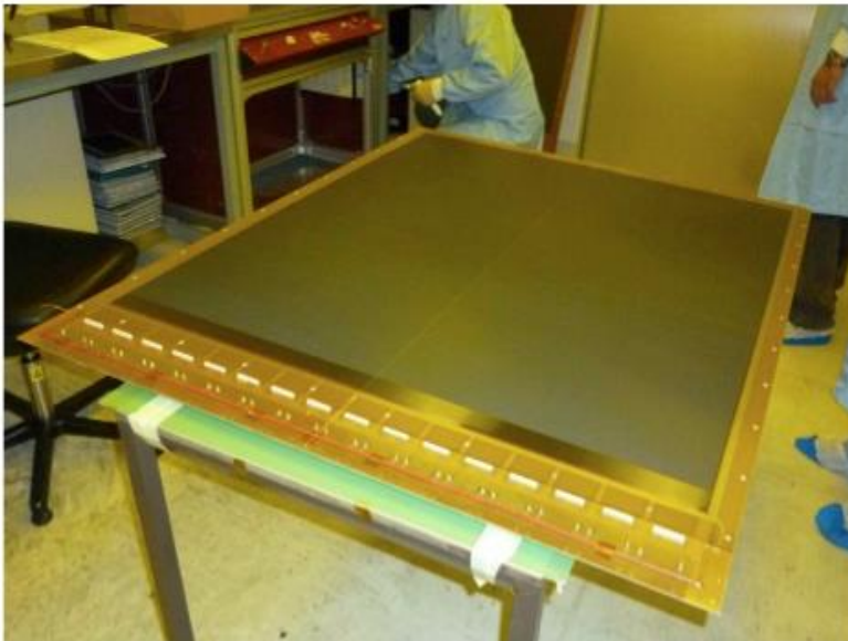
1 x 1 m 2 readout board composed of 2 boards of 0.5 x 1 m 2 2048 strips of 1.06 m length with a pitch of 0.45 mm
