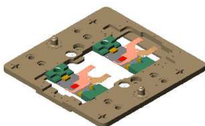
3. Two Blade B's inserted in turnplate aligned by small touch bearings
