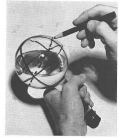
This flask has been marked with the grease pencil to indicate the celestial equator and the ecliptic (dashed), as well as four hour circles (solstitial and equinoctial colures). Pencils of different colors may be used to distinguish these and other features, and to show the sun, planets, and stars. Photo by J. E. McDonald.
