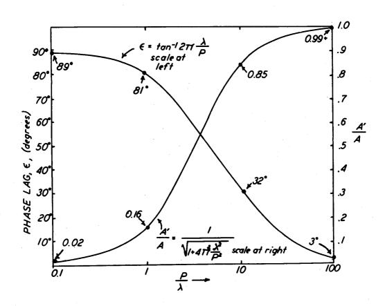
Middleton (1947, p. 62) suggests that most sensing elements exhibit a u<sup>-n</sup> dependence of lag-time upon wind speed u, so this hypothesis was checked by means of a semilogarithmic plot of the experimental data and the relation
