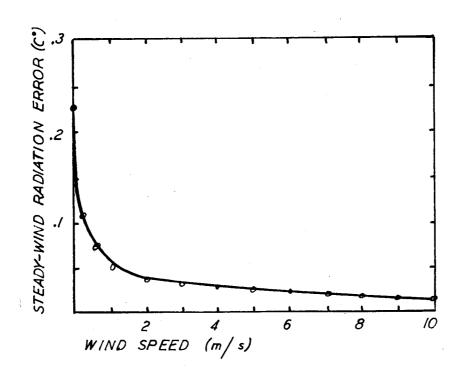
still-air conditions, very much lower than those of the bead thermistor under adverse summer conditions, as may be seen by comparing Figure 17 with Figure 9. For all wind speeds above 1 meter per second, the 0.0025-centimeter diameter thermocouple appears to suffer an error of less than 0.05 C°. Even for the very slight air motion of 0.2 meters per second the error becomes only a little more than 0.1 C°, and the still-air error itself is only 0.23 C°.
